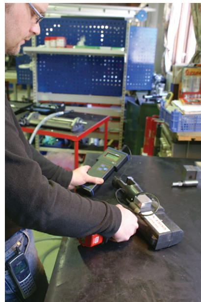
Elpress service department, calibration of crimp tool PVL1300.
