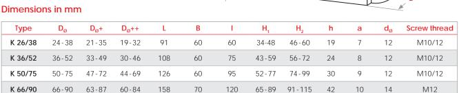
Outer cable diameter D<sub>Ø</sub>+: ~ with one Elastic Inlay Da++: ~ with two Elastic Inlavs H.
