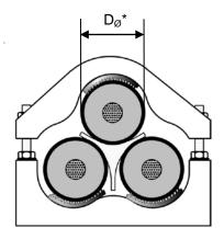
$D_{\ensuremath{\varnothing}\xspace}$  outer diameters of the single cables using Distance Wedge and Elastic Inlays
