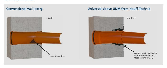
With conventional wall entries in double plug-in sleeve design, the "flow direction" is interrupted when the spigot of the underground sewer pipe (KG pipe) is inserted on the outside of the building. This can cause an "abutted edge" if there are slight settlements which cannot be entirely eliminated in the area around the working space. The result: deposits form on the edge, which, over an extended period of time, can lead to a blockage in the waste water system.
