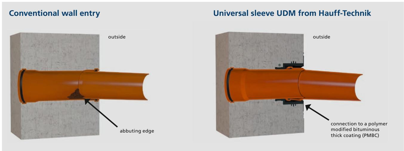
With conventional wall entries in double plug-in sleeve design, the „flow direction“ is interrupted when the spigot of the underground sewer pipe (KG pipe) is inserted on the outside of the building. This can cause an „abutting edge“ if there are slight settlements which cannot be entirely eliminated in the area around the working space. The result: deposits form on the edge, which, over an extended period of time, can lead to a blockage in the waste water system.
